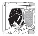
Your dryer will only function well if the filters are clean. The filters collect all the fluff which accumulates during drying and they must therefore be cleaned **at the end of each programme**, before removing the laundry, with a damp cloth. The light **Filter** is on to remind you of this operation.
