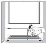
During the drying cycle or at the end, it is normal for water to be present on the surface of the condenser.
