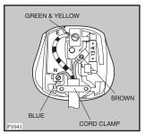
The wire coloured green and yellow must be connected to the terminal marked with the letter «E» or by the earth symbol  $\frac{1}{=}$  or coloured green and yellow.
