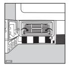
To pull out the condenser, first turn the two red stops downwards and then remove the condenser unit holding it at the handle.
