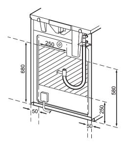
Take into account that it must be possible to pull the appliance forward sufficiently.
