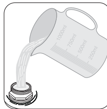
Only before filling with salt for the first time , fill the salt container with water.
