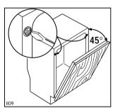
For this purpose use the two front screws. Open the door, remove the caps and screw or unscrew the screws.
