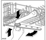
Slide out the upper basket. Push downwards on the water feed pipe, simultaneously push the spray arm upwards and turn it in a clockwise direction.
