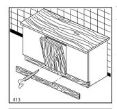
To allow correct opening of the door it is sometimes necessary to cut the kitchen plinth. Refer to the cutting table below.
