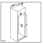
Fit the appliance in the niche by making sure that it stands against the interior surface of the unit on the side where the door hinges of the appliances are fitted. Insert the appliance until the upper strip butts up against the unit (1) and make sure that the lower hinge is in line with the surface of the unit (2).
