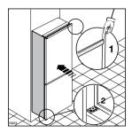
Fasten the appliance with 4 screws provided in the kit included with the appliance.
