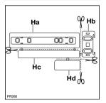
Place guide (Ha) on the inside part of the furniture door, up and down as shown in the figure and mark the position of external holes. After having drilled holes, fix the guide with the screws supplied.
