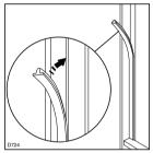
Apply covers (C-D) on joint cover lugs and into hinge holes.
