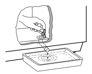
Do not try to speed up defrosting by using anything other than hot water, since this may damage the freezer. After defrosting, clean the inside of the freezer.
