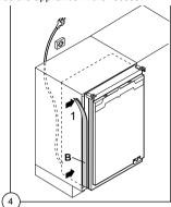
Screw appliance into place and retain the cabinet with screws (I) through the securing brackets into the worktop or adjacent woodwork as necessary.
