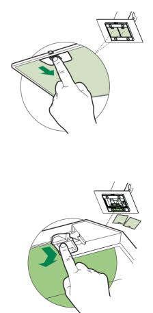
Position the new charcoal filter in the position marked and while holding the filter replace the fixing hooks as illustrated.
