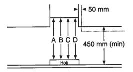
A: Built-in Electric Hob: 650mm minimum clearance
