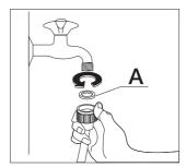
If necessary turn the hose adequately by unscrewing the nut at the rear of the appliance.
