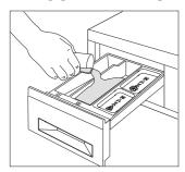
Pull the handle to open the dispenser. Enter the advised quantity of washing powder into compartment [II]
