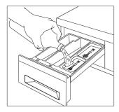
If you wish to use additives enter the softener in the compartmente with the symbol and the bleacher in the compartment with the symbol Never exceed the MAX level.
