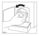
A clean filter is important for correct functioning of the washing machine, and it should therefore be cleaned regularly. Small objects left in the pockets and yarn ist retained here.
