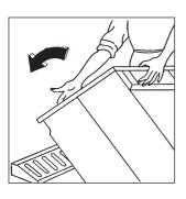
Lean the appliance back on the rear and fit one of the polystyrene angles between the appliance and the floor.
