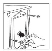
Unscrew and remove the three rear screws by means of a key.
