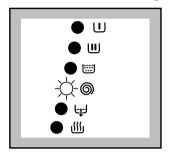
To select **Drain** press the SKIP button three times, the **wash - rinse - spin** LED,s go out.
