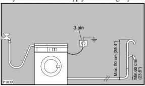
The appliance drain hose should hook into a standpipe, the hook in the drain hose is formed using the plastic "U-Piece" supplied.
