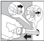
The appliance has two inlet hoses, hot and cold, with female 3/4" BSP thread connectors. If this connection is not compatible with the plumbing of the existing installation, a variety of connectors are available from good hardware stores and plumbers merchants to suit most domestic plumbing. Any alteration to your existing plumbing must be carried out by a competent person, or qualified plumber.
