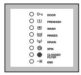
The O (Door) pilot light indicates if during the washing cycle the door can be opened:
