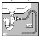
The drain hose may be extended to a maximum of 4 metres. An additional drain hose and joining piece is available from your local Service Force Centre.
