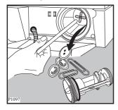
• Put the cap back on the emergency emptying hose and place the latter back in its seat.
