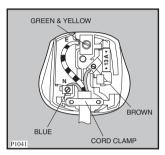
The wire coloured green and yellow must be connected to the terminal marked with the letter  $\langle E \rangle$  or by the earth symbol  $\perp$  or coloured green and yellow.
