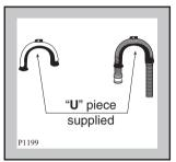
Place the drain hose into your standpipe, which should have an internal diameter of approximately 38mm thus ensuring there is an air break between the drain hose and standpipe.
