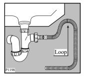
The drain hose may be extended to a maximum of 4 metres. An additional drain hose and joining piece is available from your local Service Force Centre. The joining piece must have an internal diameter of 18mm.
