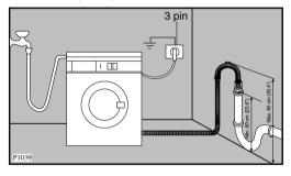
The drain hose may be extended to a maximum of 4 metres. An additional drain hose and joining piece is available from your local Service Force Centre. The joining piece must have an internal diameter of 18mm.
