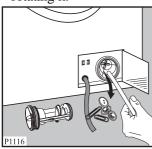
• Put the cap back on the emergency emptying hose and place the latter back in its seat.
