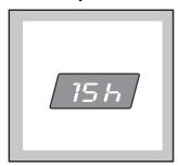
The delay time is displayed for 3 seconds, then the duration of the selected programme reappears. After you have pressed the Start/Pause button, the countdown begins, and the delay time value decreases by one unit every hour.
