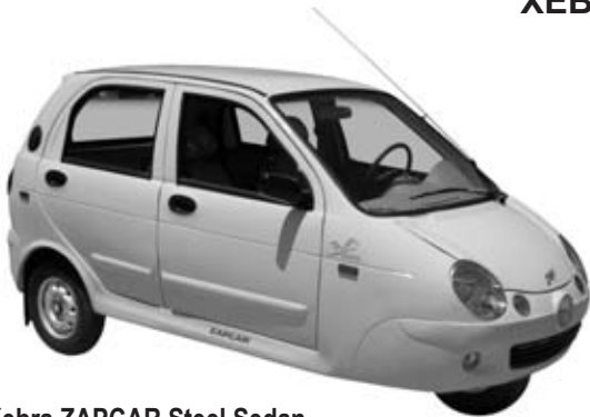
Xebra ZAPCAR Steel Sedan Length: 10.3 feet Width: 5.3 feet Height: 5.3 feet Weight: 1441 lbs. (without fuel) Gross Vehicle Weight: 2805 lbs. Charger: Universal Changer on board Classification: Zero Emission Vehicle
