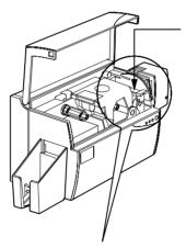
**2.** Open Printer cover and remove the yellow reminder tape from the location for the Cleaning Cartridge.
