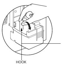
To remove, pull hook back, and lift hopper out.
