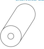
Your P310i Printer also has a Card Cleaning Cartridge. This item cleans the cards entering the printer. To ensure print quality, the cleaning roller requires periodic replacements.
