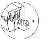
1. Install Card Cartridge by hooking onto printer as shown and clicking down.
