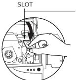
6. To replace Cartridge into printer: Make sure the arrow on top of the assembly is facing toward the rear of the printer. Hook assembly into slot on printer and rotate down. Ensure the assembly locks in place.
