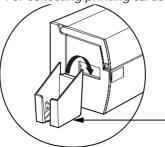
Install Card Output Hopper onto printer by hooking over bottom edge of card exit aperture.
