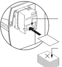
For one-at-a-time printing, feed cards through slots on side of Feeder.
