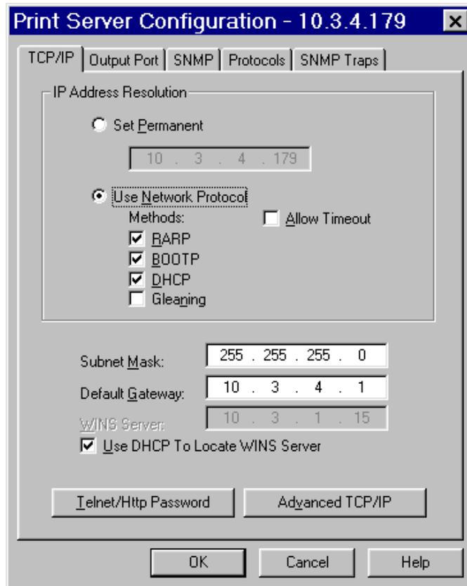
6. Type a new IP address in the text-box illustrated above.
