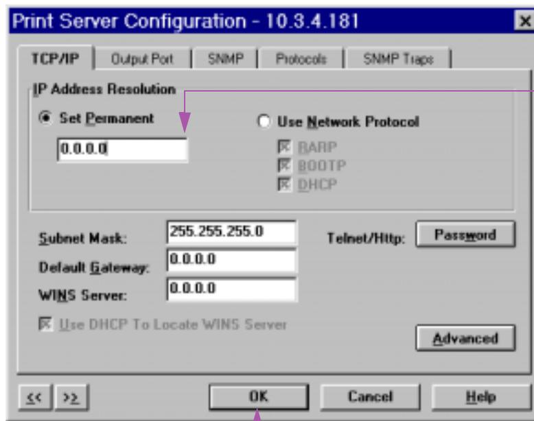
In the Set Permanent text-box, type in the print server's IP address
