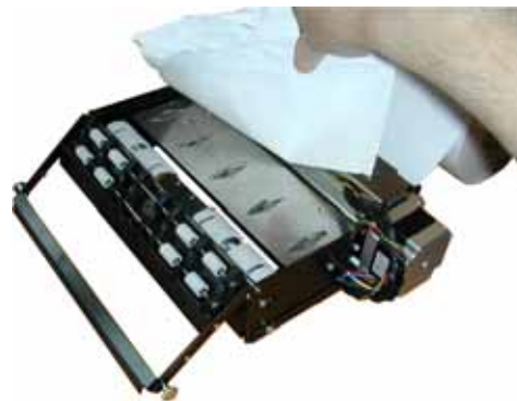
Figure 16 • Tear off the jamming paper against the fixed cutter blade.
