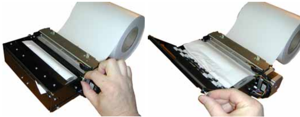
Figure 16 • Tear off the jamming paper against the fixed cutter blade.
