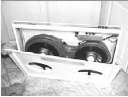
1. Remove all contents from box. Unscrew and remove bottom grease splash shield.
