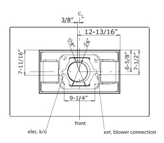
■ The following instructions are for installing the internal blower. CAUTION: To reduce the risk of fire and electric shock, install this range-hood only with internal blower models MT-020 provided with the kit cod CBI-600A.
