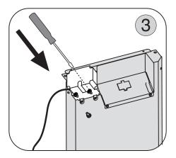
5. Connect the plate and the motor, on the remote motor support bracket, securing it using the (2 type B) screws. Fig. 5
