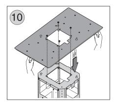
2. Secure the top support frame to the duct cover ceiling bracket by using the (4 type B) screws. Fig. 10 (11)
