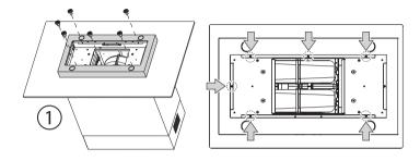
B - Take out the spacer, by removing the (6) plus (4) metric screws and the bushes. Fig. 2
