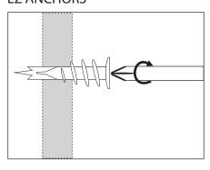
Tap EZ anchor tip into marked drywall locations, turn with screwdriver until seated flush.
