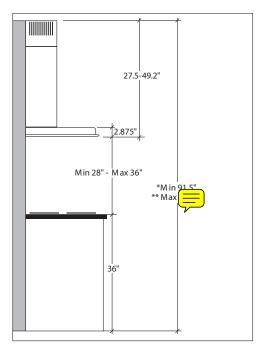
Minimum mount height between range top to hood bottom should be no less than 28".
