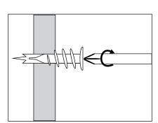
Note: Whenever possible, the hood should be secured to wood studs celling and/or wall with minimum thickness 3/8".
