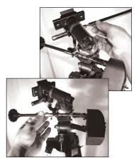
6. Tighten all setscrews on the mount assembly to prevent movement of mount. Tighten the set screw on the counterweight to prevent movement of weight on balance shaft. Screw threaded end of balance shaft into the threaded receptacle opposite the telescope mounting bracket on the upper part of the mount. Tighten balance shaft for stability.
