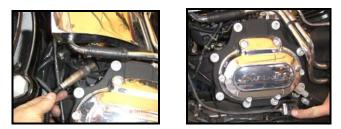
**ST-E:** Position the harness plug for the front pipe under the transmission, along the frame rail. Install the oxygen sensors into the exhaust pipes, connect the harness plugs to the oxygen sensors and secure the harnesses to the frame (above the lowest point) with wire ties.
