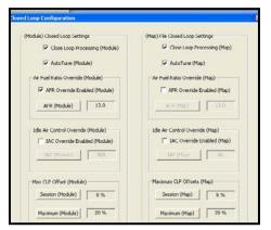
The Closed Loop Configuration dialog page opens; the right side shows the default MAP settings stored in the MAP file (settings are applied to the installed base map during the 'Closed Loop Format' conversion performed by SmartLink), while the left side shows what the module is currently set to (unadjusted, these settings will mirror MAP's settings).
