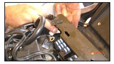
**ST-C:** Connect the ThunderMax ECM to the harness and position it loosely in the ECM tray. Feed both oxygen sensor harnesses (front cylinder first) through the gap between the frame and oil tank on the right side of the motorcycle.
