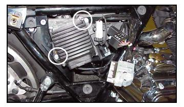
**FL-C:** Install the ECM wiring harness to the ThunderMax ECM. Do not install the ECM onto the motorcycle at this point. If the ECM is mounted onto the electrical caddy at this step, it is difficult to get the fuse box in place.
