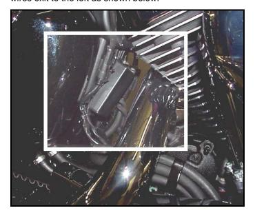
**Step 2d** Insert AutoTune power/communication 4-pin plug into the bike's data port (gray), located at the base of the battery, left side of the bike.
