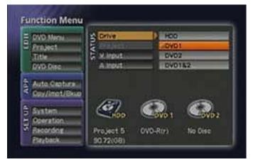
Although the hardware is connected for Composite, the Video Input source must also be set to Composite. From the **Function** menu, highlight **V** Input from the Status window then press **Enter**. Arrow right to highlight **Composite** then press **Enter** so that the option is marked with an orange box (**=**).
