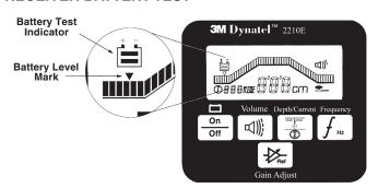
To test the batteries, turn the Receiver on by pressing and holding. The bar graph should extend to the right of the battery level mark, otherwise replace the batteries.
