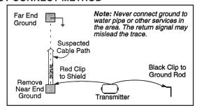
Make sure the Transmitter is off. Plug the Direct Connect Cable into the front panel jack. Connect the Black clip to the ground rod. Place the ground rod in the earth perpendicular to the suspected cable path. If necessary, extend the black lead with the Ground Extension Cable. Next, remove the ground bonding and attach the Red clip to the shield.
