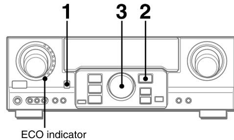
Setting this unit to the ECO mode reduces power consumption as below.
