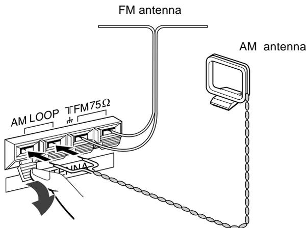
**To stand the AM loop antenna on a surface**
