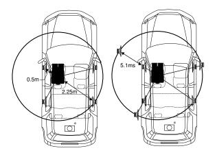
Here we calculate the time correction value for the front left speaker in the diagram at the left. Conditions:
