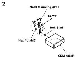
When your vehicle has the Bracket, mount the long hex bolt onto the rear panel of the CDM-7892R and put the Rubber Cap on the hex bolt. If your vehicle does not have the Mounting Support, reinforce the head unit with the metal mounting strap (not supplied). Connect all the leads of the CDM-7892R according to details described in the CONNECTIONS section.
