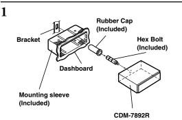
Remove the Detachable Front Panel (refer to page 4). Slide mounting sleeve from main unit (see Removal Procedure below). Slide the mounting sleeve into the dashboard.
