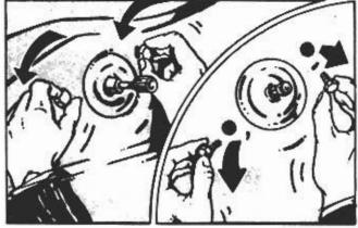
B · AFTER REMOVING ORIGINAL BOLTS FROM THEIR SEATS, REFER TO THE TABLE BELOW TO CHOOSE SUITABLE SPACERS AND BOLTS (SUPPLIED IN KIT No. 2).
