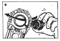
Geared sleeve to be inserted towards inside of vehicle
