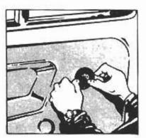
Place adhesive over pivot making sure that it adheres properly to door casing
