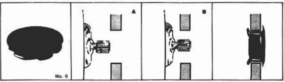
When the regulator pivot does not come out from the panel (photo A and B) you can use cap No. 0 for a better appearance.
