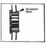
The grommet has to come through the door casing at least 5/32 in order to be locked with the retainer ring.
