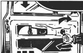
Adjust the registers or guides if the window does not operate freely
