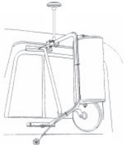
Figure 5. Mirror Mount Cable Routing
