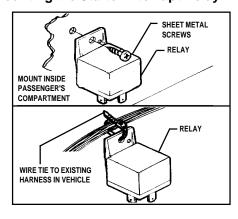
The relay will be mounted in the passenger's compartment. Mount the relay close to the wires from the ignition switch.
