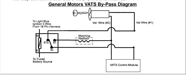
5. Connect the previously selected resistor from terminal #87 to the second (#2) wire (as shown). **NOTE:** The above information and following diagram is for the GM VATS system only. For GM PASS LOCK System you will require the Audiovox AS-PASS II Module.
