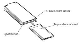
To remove the PC CARD, press the Eject button. The button will pop out. Press the button again until you hear a clicking sound. This will eject the PC CARD.
