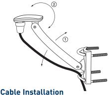
At this point you are ready to attach the RG6 coaxial cable (sold separately). Take either end of cable and insert it through the rubber boot then screw the connector onto the bottom of the antenna as shown below. Screw the connector on by hand as far as it can go. It is not necessary to use any special tools for this.
