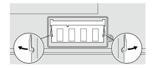
8 Align the notch in the contact edge of the SO-DIMM with the divider in the socket. Firmly insert the SO-DIMM into the socket at an angle of 20 degrees , and then pivot it downward until it snaps into place 2.
