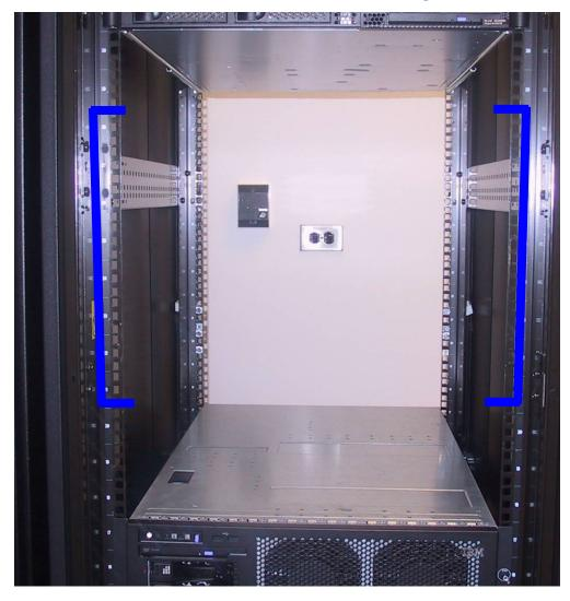
The length of the scalability cables requires that no empty U-spaces exist between the nodes.
