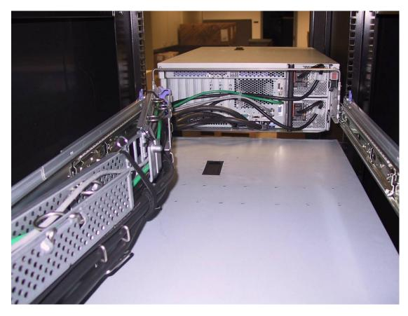
Once all cables are secured in the CMA, pull the system out all the way and pull the scalability cables tight within the CMA hanger brackets. Retighten the cable straps if needed. This will ensure the cables stay in the CMA while sliding the system in and out for hardware maintenance and upgrade activities. This is especially important because thinner cables are used in this M2 generation of the x3950 system compared to the previous version.
