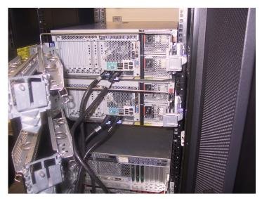
Connect cables to scalability ports according to the system manuals.
