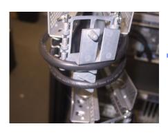
Route cables through hanger brackets, balancing the slack in the cables between the CMAs and the nodes and in the side of the rack.
