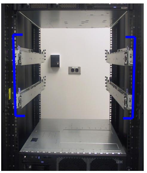
Use Rack Installation Instructions manual to space slides appropriately and install the slides into the rack. Note this system is 4u as opposed to 3u for the original System x3950/xSeries 460.
