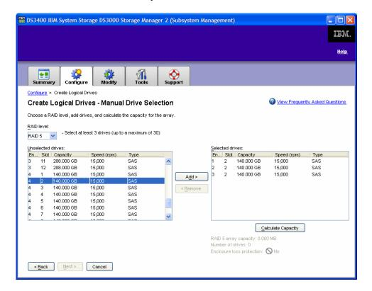
Once all the drives are selected, select **Calculate Capacity** to ensure the proposed array will be your capacity and channel protection requirements. Then click **Next**.
