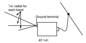
$1/4\lambda$  (quarter wavelength) radial for each band is suitable for a counterpoise. Install the counterpoise directly below the AT-141's ground terminal. Insulate the ends of each radial from other metal objects. Layout the radial horizontally and as straight as possible.
