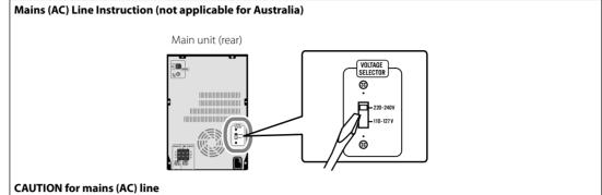
BEFORE PLUGGING IN, do check that your mains (AC) line voltage corresponds with the position of the voltage selector switch provided on the outside of this equipment and, if different, reset the voltage selector switch, to prevent from a damage or risk
