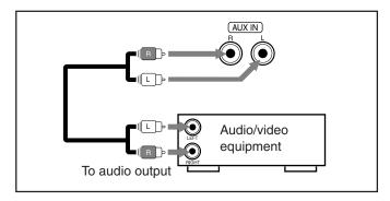
For playing the other equipment through this unit, connect between the audio output jacks on the other equipment and AUX IN jacks by using audio cords (not
