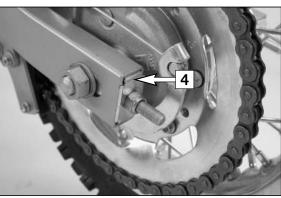
To mount the wheel reverse the procedure described above. Always hook the brake backing plate into the swing arm support.
