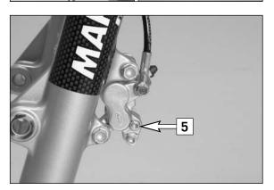
Mount the left brake shoe and fix with screw. Mount the right brake shoe and tighten the screw to 4 Nm. Mount the lock washer. Align brake shoes, mount front wheel (see chapter: Mounting the front wheel).
