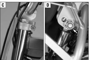
Figures C and D show the fork and shock absorber positions for a high seat position. Fork tubes are plane with top of upper fork stabilizer. (Screw cap (Aluminium) protrudes from the top of the upper fork stabilizer)
