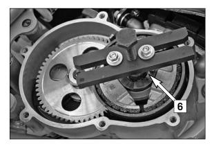
Screw the extractor (special tool item no. 590.29.021.044) onto the clutch hub [6] with the M5x50 screws, hold the extractor and remove the centrifugal clutch from the crankshaft by screwing in the extractor screw. Completely remove the centrifugal clutch, bearings and spacing washers from
