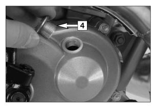
Remove stopper [4] and fill in 0.15 liters of automatic gear oil (Motorex ATF Super). Mount the stopper and check the engine for tightness.
