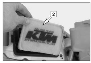
Thoroughly wash the foam filter in special cleaning fluid (Motorex Bio Dirt Remover) and allow it to dry well. Only press out the filter, do not wring it out under any circumstances. Oil the dry foam filter with a high-grade filter oil (Motorex Liquid Bio Power). Also clean the air filter box. Check carburetor collar for damage and that it is filled correctly.
